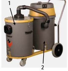
The motor top must not be covered when the machine is operating. If the air current from the suction motors cannot leave the machine there is a risk of the motor top being overheated and damaged.
