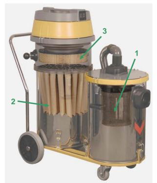
A strong wire grating (1) in the cyclone separator in container 1 holds back the large particles, and because of the cyclone effect in the container also a large part of the small particles will be held back. In container 2 the large multi-tube filter (2) is made of a fire-resistant filter material.
