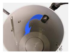
The collection container has also diversion for static electricity, and the oblique container connection piece ensures the cyclone effect in the container.
