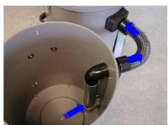
The suction pipe ending near the bottom of collection container 1 will draw the filtered liquid from container 1 through the connection hose to container 2.
