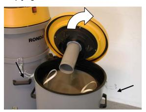
The collection basket in container 1 keeps back the large particles and is emptied when needed. When the collection basket is almost full, the vacuuming is stopped. Let the machine empty container 1 of any liquids before the machine is switched off.
