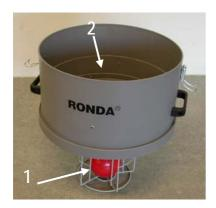
The motor top is mounted on an adaptor ring and is secured with two container clips. The float valve (1) mounted under the adaptor ring blocks the air current if the collection container is filled to overflowing. In this way the suction motors are protected against water being sucked up into the motors.
