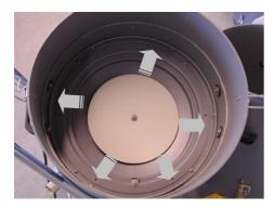
In the liquid/dust separator the air current will hit the stop plate. This lowers the air velocity as the air current is conducted round the stop plate.
