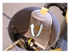
Release the filter bag from the connection piece of the container.
