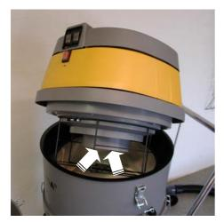
The purified air current is drawn up through the suction motors in the motor top.
