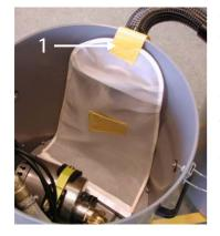
The fine-meshed filter bag is mounted on the connection piece in container 2. The yellow support patch (1) carries the filter bag, and holds it over the connection piece while the filter bag is being filled.
