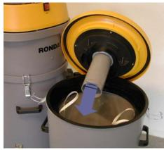
The liquid is led through the guide pipe, which will hold back all the large particles, chips etc.
