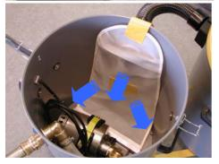
The fine-meshed filter bag will hold back the small particles. The cleaned liquid will run through the filter bag and will gather in container 2.
