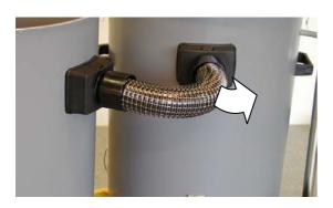
Remove the suction hose, which connects the two containers.
