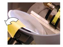
• Make sure that the support flap of the filter bag folds over the container edge. The support flap will help carrying the filter bag.
