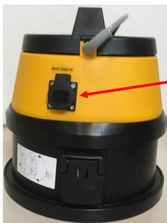
The automatic start/stop is programmed for delayed motor stop. Therefore the suction will continue for some seconds after the hand tools has been switched off before the machine will stop.
