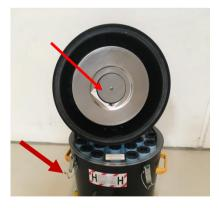
Loosen the four container clips of the motor top and remove the motor top. Place the motor top so that the filter is easily accessible.
