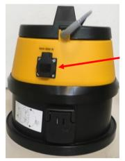
The automatic start/stop is programmed for delayed motor stop. Therefore, the suction will continue for some seconds after the hand tools has been switched off before the machine will stop.
