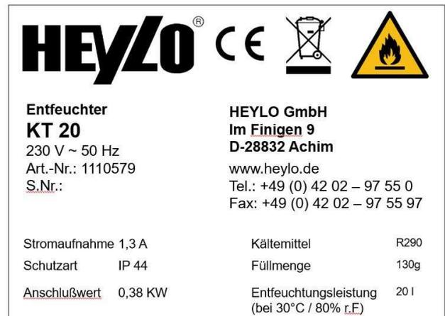
Fig. 10: Rating plate (example illustration)
